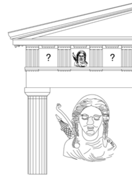
Fig. 5. Reanimation of 027.101 triglyph-metope and the Artemis figure on it in the superstructure of the virtual Archaic Artemis Temple in Doric order (S. Akin - Ö. Ürkmez)
